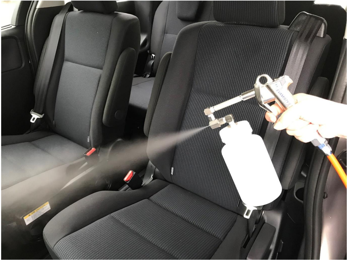
Eva-Mist disinfecting the interior of a car
